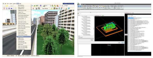
Figure 4a,b - Import/export IFC menu; an IFC file opened in 3D Cad
